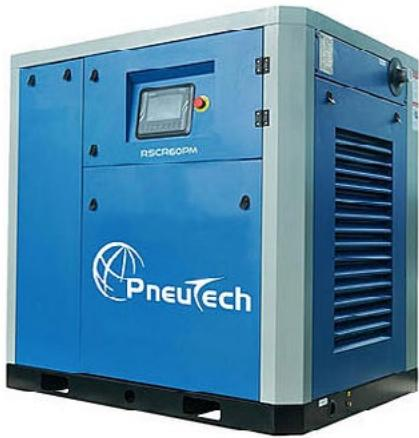
The PneuTech PM series air compressor uses a permanent magnet and variable speed drive technology to seamlessly speed up and slow down, or even completely stop, the compressor to match your air demands. After 60 seconds of no air demand the motor simply stops. When installed in a business with an air demand that varies throughout the day, the savings can be significant – as much as 60%!
